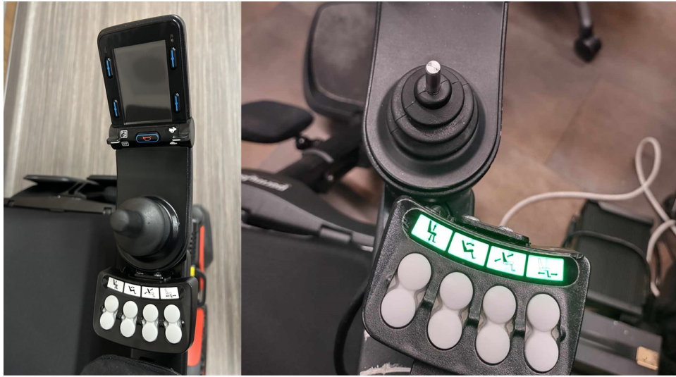
Fig. 1. An example of the number of buttons needed to control the tilting of a power wheelchair
